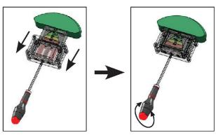
Pre-tension the tensioner using the screws situated under the body
