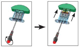
The springs can be loosened to the tension required starting with the one in the middle, leaving the belt (or chain) under pressure. There are two different types of springs.
