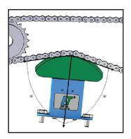
Once the angles of the belt or chain are equidistant to the tensioner, manually put it under tension and tighten.
