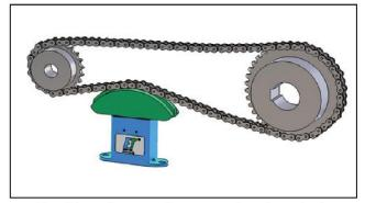
Position the tensioner under the chain (or belt) as close as possible to the sprocket on the slack side
