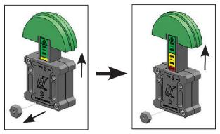
The spring can be released by removing the pre-tension button, thus freeing the tensioner
