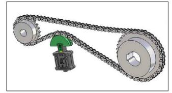
The tensioner is now ready for use. The stroke of the tensioner should be within the green range.
