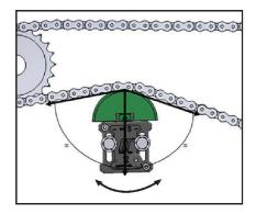
Once the angles of the belt or chain are equidistant to the tensioner, manually put it under tension and tighten.
